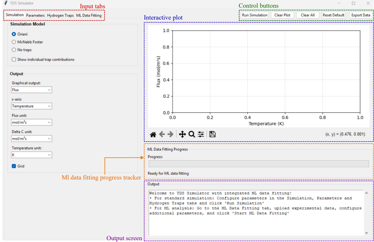
Figure 1: GUI upon launch, highlighting key components. The default configuration loads the "Novak_200" case, which contains all parameters as published in the associated manuscript.
